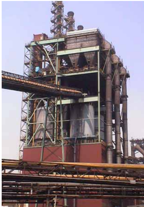
Sistema P.C.I.(Powdered Coal Injection)
